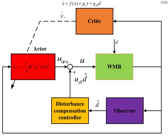
Figure 2: Control structure diagram III. Controller Design for WMR
